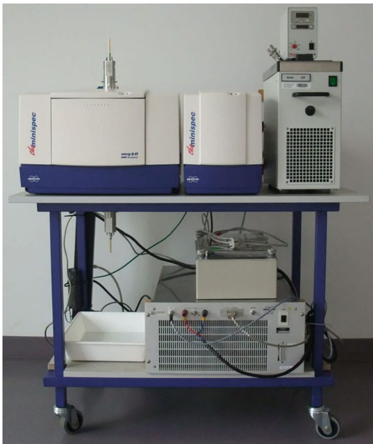
Fig. 3.4 Compact and mobile low-field system for the NMR-based capillary rheometer. The height of the magnet box on the left of the table amounts to 0.32 m without the aluminum parts at the ends of the flow loop, see Sect. 3.4. In the middle of the table the electronic box can be seen. A cryostat used for thermostating of the flow loop is placed on the right. The 60-A gradient amplifier and the electronics for pressure-difference and temperature recording are located on the lower board
