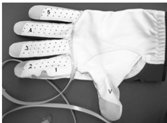
Fig. 2. Five channel real-time MIDI-Glove. When electrical contacts 1-5 contact electrical contact V, a closed electrical circuit is created.
