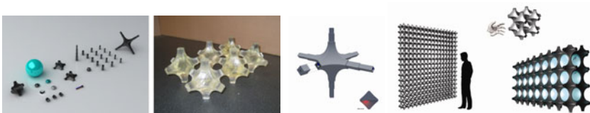
Fig. 4. This module used a six-pointed star with linear actuators on extending arms for motion and latching and a strategy for injection infill
