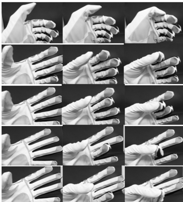
Fig. 1. The five different hand movements associated with the MIDI-Glove. Each row illustrates hand postures related to playing a unique note.
