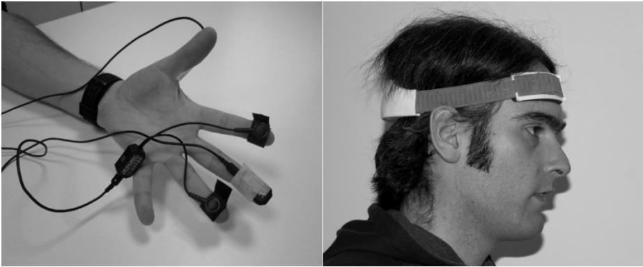
Fig. 2. Devices used for the final comparison test with user involvement: Procomp Infiniti hands sensors (left) and our last prototype of headset (right)
