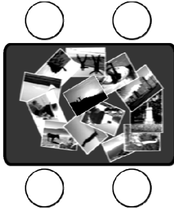
Fig. 2. An example of the visualization of a collection of pictures on a multitouch tabletop display with four users around it. The spiral organization and the random orientation of the pictures puts all the users in an equal position for browsing through the collection.
