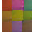
Fig. 3. 3x3 grid depicting skin under different projected light as seen by onboard camera. The wide color gamut makes skin-tone detection based methods ineffective.
