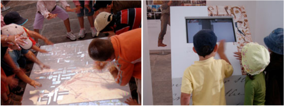
Fig. 2. The interactive floor about the transportations' culture (top) and the virtual book, which can be browsed by page-flipping gestures performed in mid-air (down)
