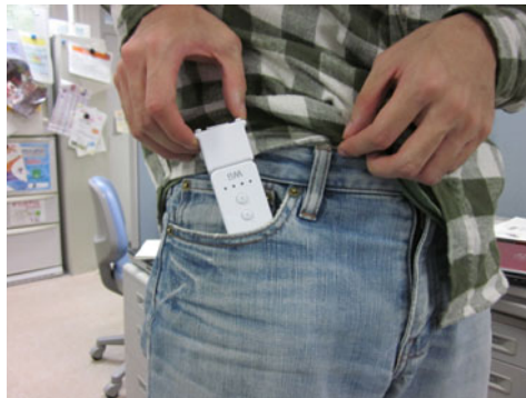
Fig. 1. Appearance of sensor position. We plan to activate incident detection application only when mobile phone is in bottom of user's pocket. Bottom of user's pocket can be expected not to have considerable individual difference in shape.
