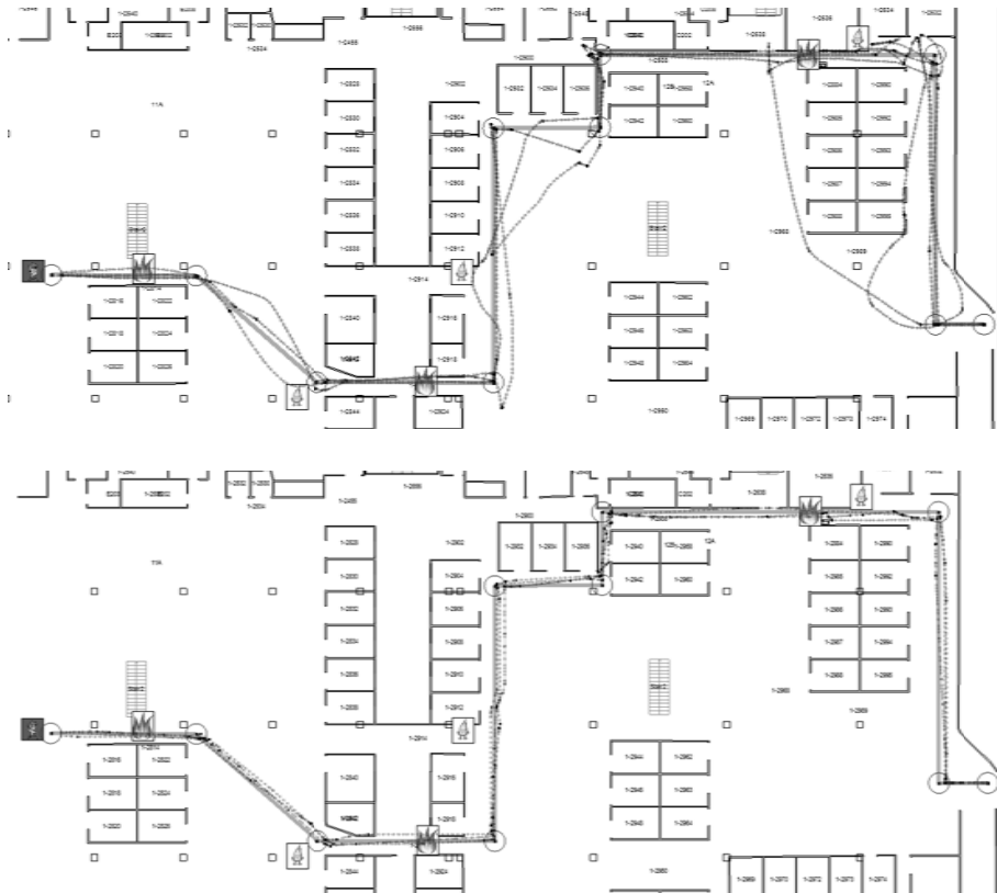
Fig. 1. Examples of recovered walking traces along one of the routes in high visibility (upper) and low-visibility (lower) conditions, both with the speech display mode. The thick solid line indicates the planned route. The thin dotted lines indicate walking traces of three participants. The participants started from the right end of the route to rescue the person that was at the left end of the route (dark icon). The icons along the route indicate fires. The circles at each waypoint cover the range of its capture radius. If the walking trace did not get through the circle around a waypoint, then this waypoint was regarded as a missing waypoint.
