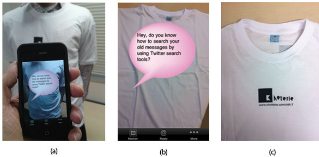
Fig. 3. (a) User using this application to recognize AR marker, and the latest Tweets will be presented. (b) The interface layout design. (c) The AR marker is printed on T-shirt on two sides.
