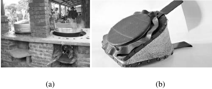
Fig. 1. (a) Traditional method of blowing for fire (b) wind-blower
