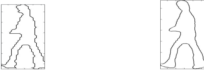
Fig. 3. Human Silhouette Representation. (a) Is the silhouette representation using all the Fourier Descriptor terms (i.e. 200 terms for the given example) and (b) is the silhouette reconstruction using 60 terms.
