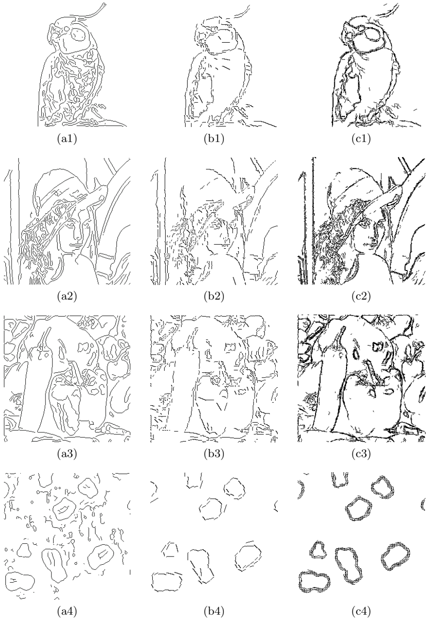
Fig. 4. Examples of edge detection: (a) Canny, (b) wedgelet transform, (c) sliding wedgelets
