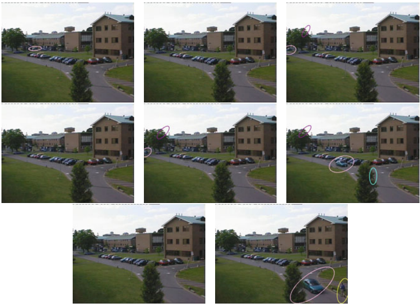
Fig. 5. Tracking object with occlusions. The algorithm can recover tracker identification over occlusions with less than five seconds (100-150 frames).
