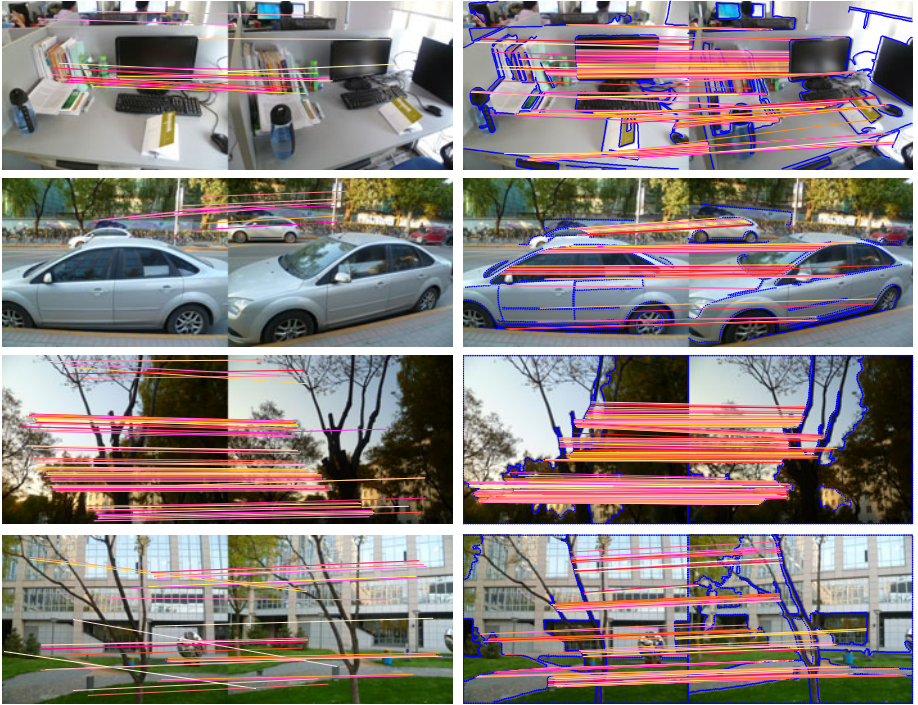
Fig. 5. Experimental results for real-world images. All the left pairs are the results of SIFT-based stereo matching. All the right pairs are the results of the proposed algorithm. Matched contour points are linked by the colored solid lines. The blue contours of the top two and the bottom two rows of images are extracted using the method of [5] and [6] respectively.
