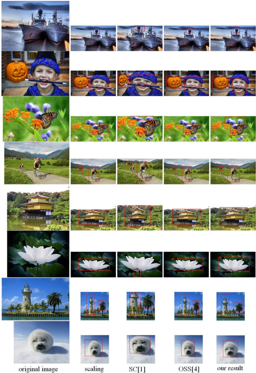
Fig. 5. Comparison of our results with those of scaling, seam carving (SC) [1] and optimal scale-and-stretch (OSS) [4]. The results of scaling, OSS [4] and our method tend to be smoother than those of seam carving. Notice the discontinuities in the ship, people, flowers, house and tower, which are caused by the pixels being removed. Compared with scaling and OSS [4], our method can preserve the aspect ratios of prominent features better.
