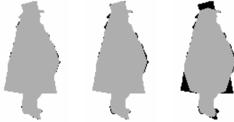
Fig. 9. From left to right, the patterns recovered by applying the reverse distance transformation to the skeletons based on \theta -CMD with \theta=5 , \theta=6 , and \theta=7 . Pattern's pixels that are not recovered are shown in black.
