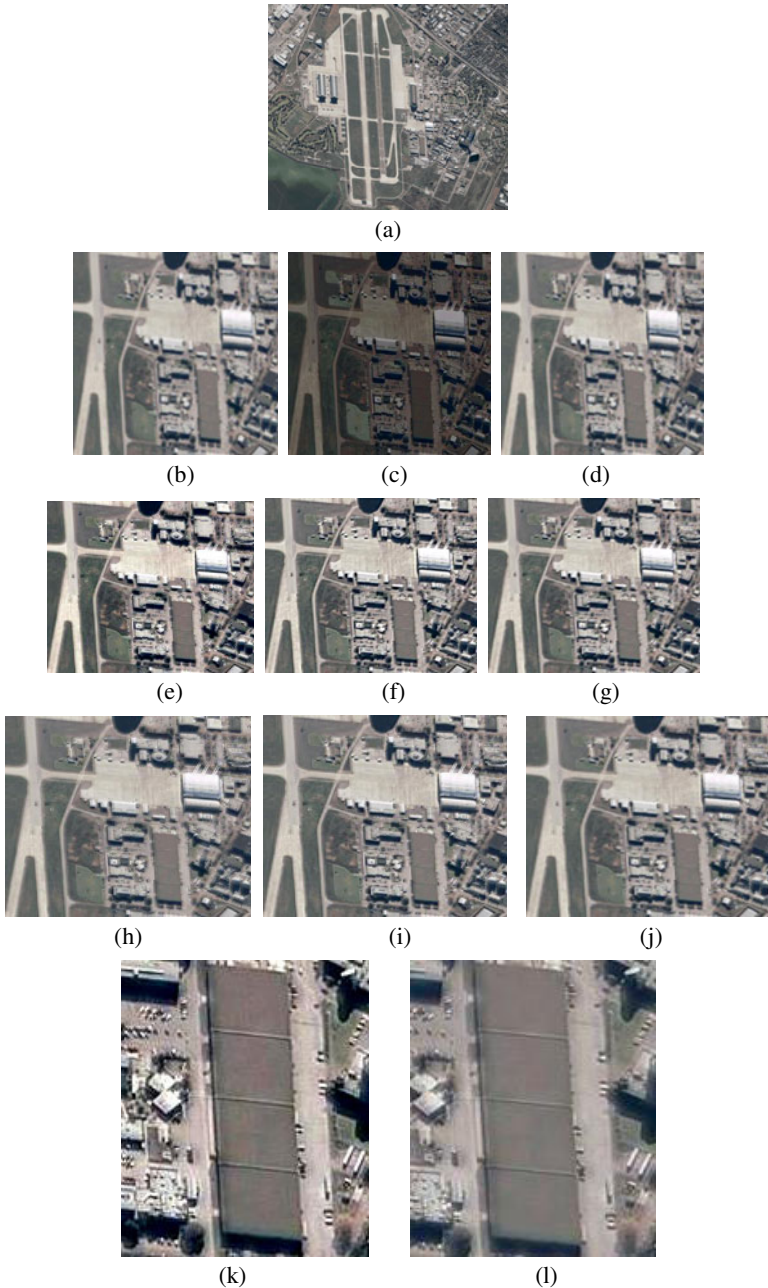
Fig. 1. Fusion of Quickbird MS image and PAN image. (a) Multispectral image; (b) Sub-image of MS image; (c) LHS fused sub-image; (d) DWT fused sub-image; (e) NAWs fused sub-image; (f) NAWRGB fused sub-image; (g) NAWL fused sub-image; (h) AWS fused sub-image; (i) AWRGB fused sub-image; (j) AWL fused sub-image; (k) Small image cut down from figure 1(e); (l) Small image cut down from figure 1(h).
