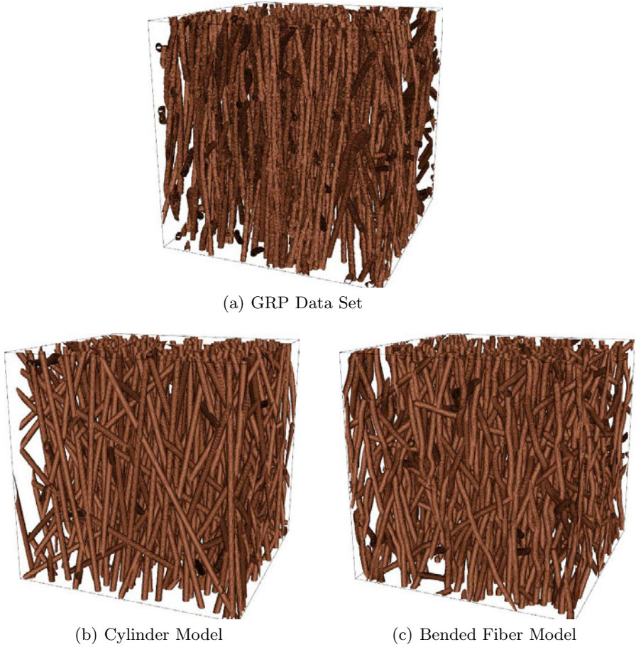
Fig. 1. Modeling of glass fibre reinforced polymer. Surface Rendering of real data set and realizations of stochastic models.
