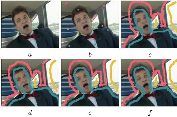
Fig. 3. Sets of markers on sequence carphone (a) frame 8 of extract from carphone sequence, b) few points on frame 8, c) heavy markers on frame 8, def) heavy markers on frame 4,8 and 11)
