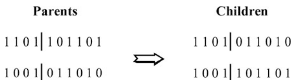
Fig. 7.4 Example of crossover operator under binary coding with one splice point
