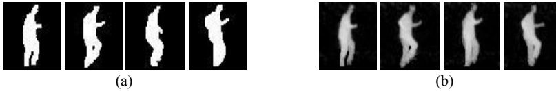
Fig. 2. Two sequences of (a) binary and (b) depth silhouettes of a rushing activity
