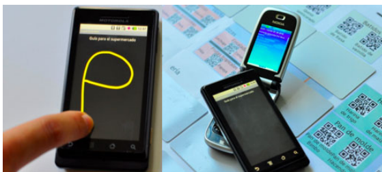
Fig. 3. User drawing a “P” (left) on Motorola Milestone, Nokia 6131 NFC to read HF RFID tag for navigation and supermarket mock-up for testing (right)
