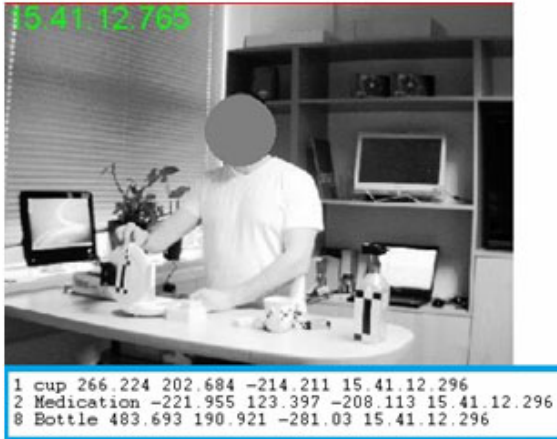
Fig. 2. example scene captured by stereo camera. Also shown is the data stored in relation of the scene. Included are object: IDs; labels; global coordinates; orientation and; timestamp.
