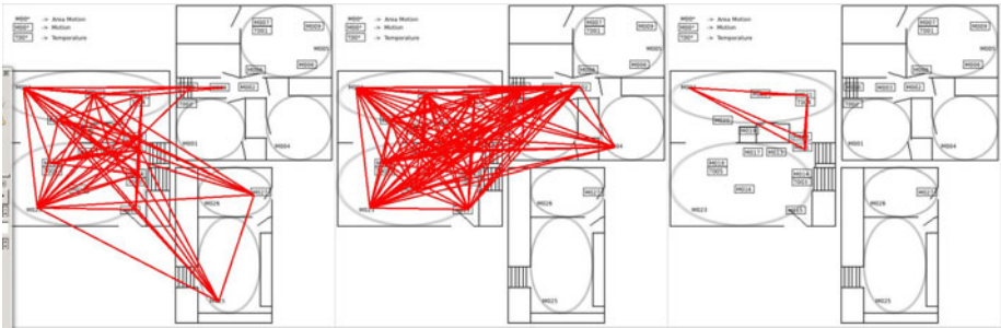
Fig. 1. The left two graphs are both of breakfast. Both include many sensor events outside the usual area of the activity. The rightmost picture is a frequent subgraph among all breakfast graphs.
