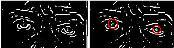
Fig. 3. Iris localization using Hough transform
