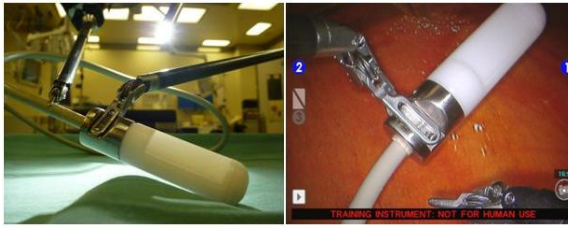
Fig. 2. The pick-up IAUS transducer is grasped and manipulated by the Pro-Grasp tool of the da Vinci Surgical System
