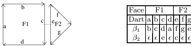
Fig. 2. Open combinatorial map example. Darts a, b, d, f and g are not 2-sewn.
