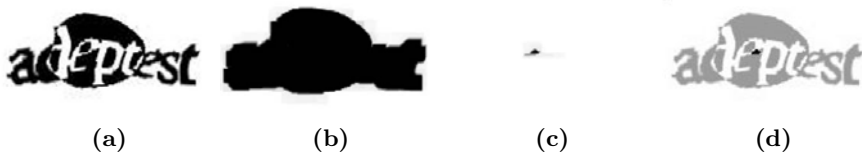
Fig. 3. Ellipse center estimation. After 7 iterations of erosion only one connected component is left (b). After 58 iterations of dilation only a few pixels close to the center are left over (c). Figure (d) shows these pixels in relation to the original image.
