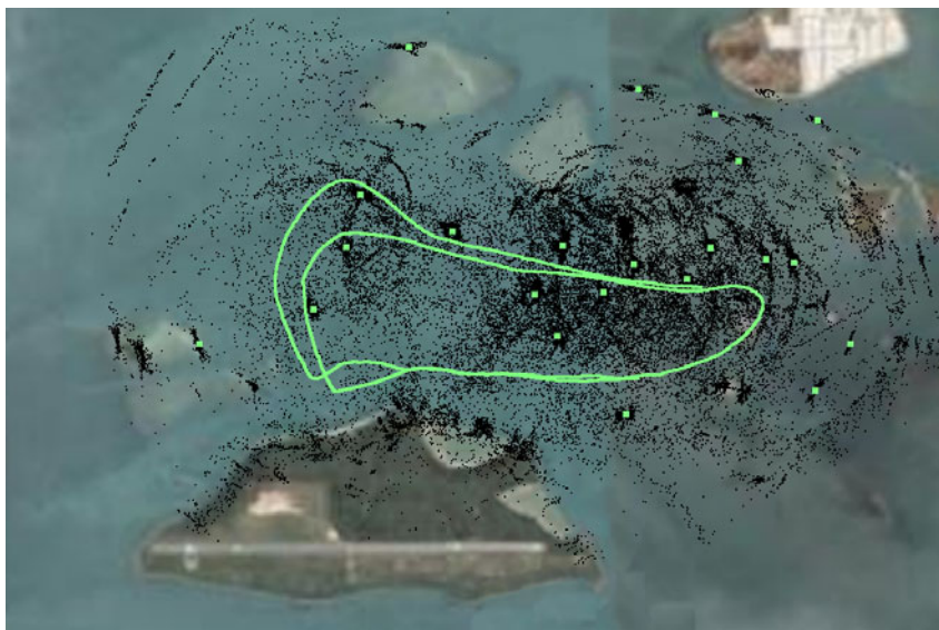
Fig. 6.15 Overview of the test site ( 1^{\circ}13' N, 103^{\circ}43' E ), showing the GPS trajectory (green line) and GPS coordinates-ordinates (green dots) of the point feature map. The point feature measurement history is also provided (black dots).
