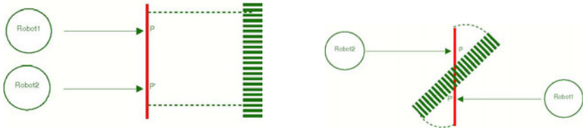
Fig. 2. Definition of states and actions. a) Decrease distance. b) P decrease, P' increase.
