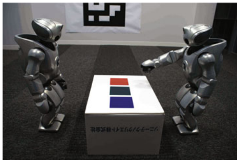
Fig. 1. Robotic experiments with the Colour Naming Game. The speaker draws attention to a chip by naming its colour and the hearer points to the chip which has been named. Agents give feedback after this interaction in order to share and align their colour categories and vocabularies.
