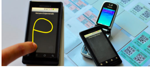
Fig. 2. User drawing a “P” (left) on Motorola Milestone, Nokia 6131 NFC to read HF RFID tag for navigation and supermarket mock-up for testing (right)
