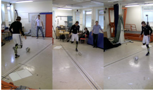
Fig. 4. A motion capture studio was used to capture ground truth animations corresponding to video from three cameras
