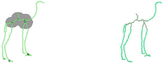
Fig. 2. The zones of influence, shown in gray, obtained by applying the reverse distance transformation to the branch points, left, and the three types of partition components, right
