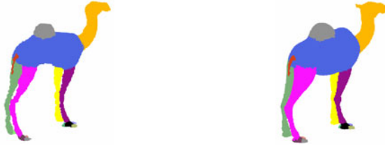
Fig. 3. Simple regions, bumps and kernels after the first recovery step, left. Decomposition of “camel” where each skeleton partition component is associated with an individual object part, right.
