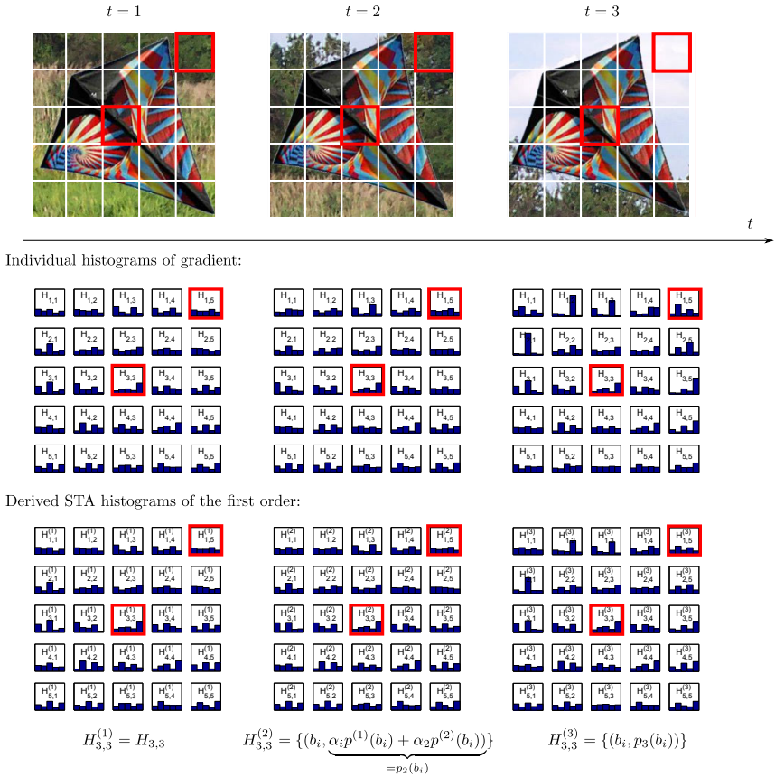
Fig. 1. Constructing the first order STA histograms for a sequence of three frames. Two patches are highlighted in red: a patch which lies in the background and a patch which lies on the object. Notice how the STA histograms of the object patch are constant through time, while the STA histograms of the background patch change.
