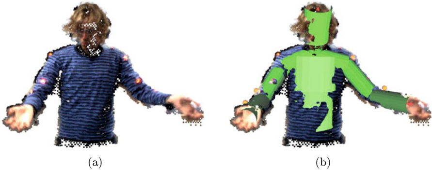
Fig. 2. (a) A segmented stereo image of a human body. (b) A human skeleton estimate projected on the image data.
