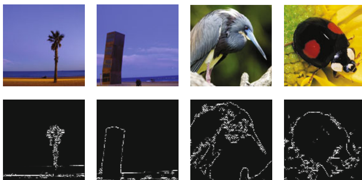
Fig. 8. Rebuilding the original pictures in an 100 \times 100 square from SC-like neurons output. Each rebuilt picture is actually composed of many linear segments.
