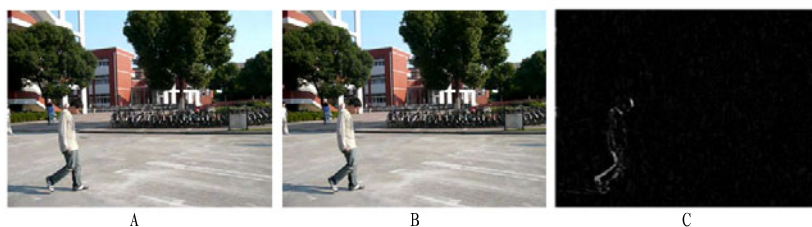
Fig. 2. An illustration of phase discrepancy. A and B: Two adjacent frames. C: The motion saliency map of A and B using phase discrepancy.
