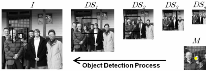
Fig. 2. Face detection process after down sampling an input ( I ) image. In each down sampled ( DS ) image, 64 \times 64 pixel size windows (for example, solid squares in the DS_1 , DS_2 and DS_3 ) are set up to search the most likely pixel position of the model ( M ) face. A filled circle is an extraction point for the M face. After the process, our Gabor pyramid system can detect the M face on the image I with a small frame of 20 \times 20 pixel size.
