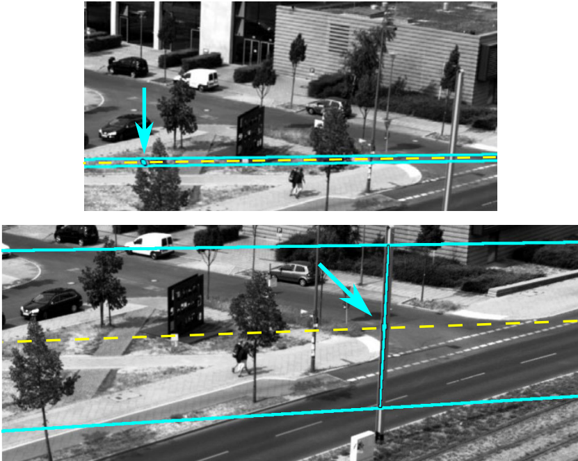
Fig. 3. Classic Matching: Wrong Correspondences due to Center Constraint only. Two features were matched by classic epipolar line matching (see yellow/dashed epipolar lines). This correspondence is wrong but would have been ruled out by the tangent epipolar lines, as becomes obvious in these images (blue tangent epipolar lines).
