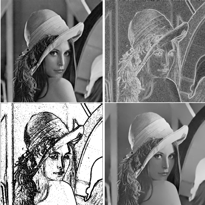
Fig. 2. Top: Left: Original Lena image; Right: Singularity exponents estimated using the Local Correlation Singularity Measure; they are represented using a inverse grayscale palette (the brightest the smaller, so more singular). Bottom: Left: MSC, defined as \{h < -0.5\} ; it comprises 30% of the points of the image ; Right: Reconstruction. Some details are missing due to the lack of capability of the method to capture every UPM point; however, the reconstruction is of high quality (24.5 dB).
