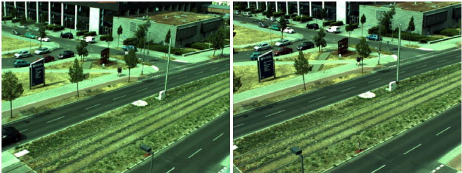
Fig. 1. Outdoor Data Set. The input images are a stereo image pair from an outdoor scene. The baseline is \approx 6.7 m and the distance to the scene somewhere between 20 m to 100 m. The scene contains natural areas and man-made structures (i.e homogeneous and repeating parts).
