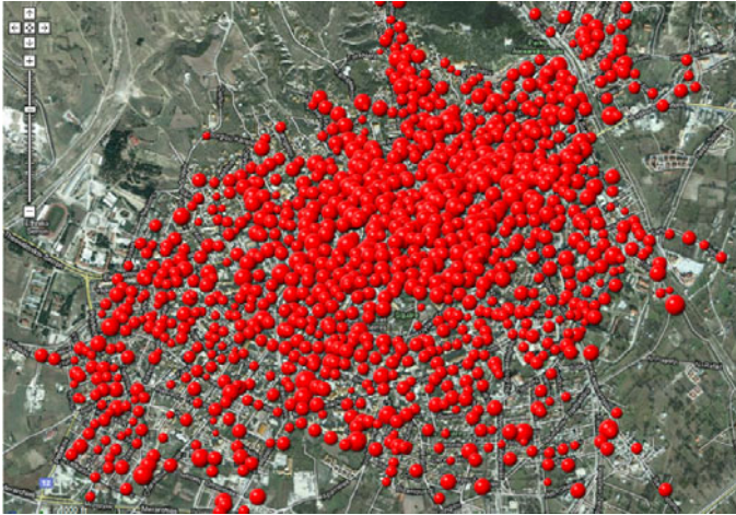
Fig. 2. Wi-Fi coverage of the city. Measured SNR values are visualized by the size of the sphere.
