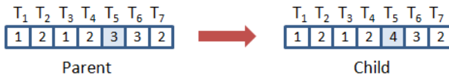
Fig. 10.6 The Mutation operation: A task is randomly selected in a chromosome. An alternative service which is also capable of executing the task is randomly selected to replace the current task allocation
