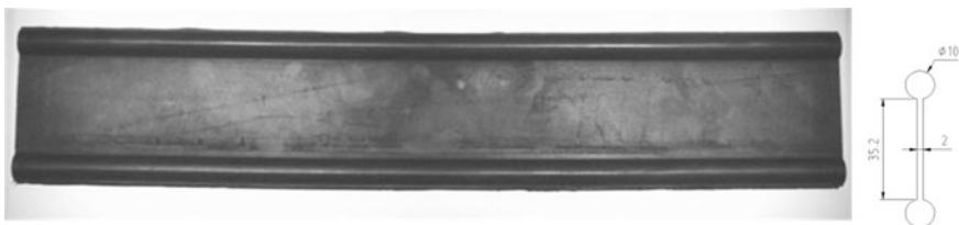
Fig. 57 Pure shear specimens for crack growth tests
