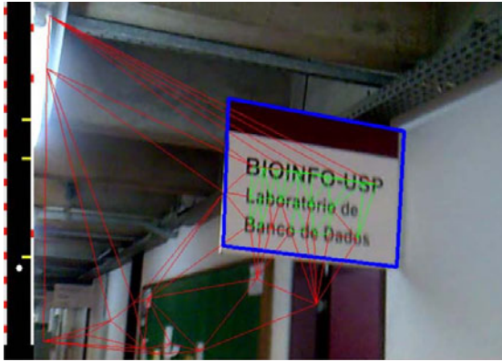
Fig. 5. User interface shown by device. The white dot on the left represents the user position in the corridor.
