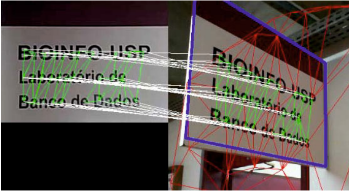
Fig. 4. Example of detection using keygraphs. The white lines between the image on the left and right shows the correspondences found. Green triangles on both images shows the keygraphs matched, and red ones on the image on the right shows keygraphs not matched. Blue bounding box indicates estimated pose.
