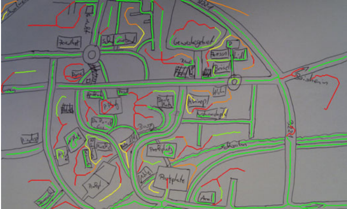
Fig. 4. Line segments colored by their ratings. Rating less than 0.5 (red), less than 0.75 (orange), less than 1 (yellow), less than 1.5 (light green) and 1.5 and greater (green).
