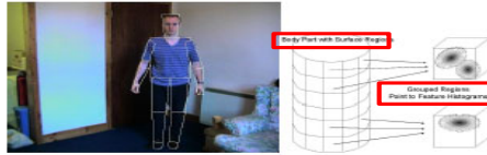
Figure 1. An articulated body model with feature distributions defined over surface patches. These patches are grouped based upon similarity and knowledge of clothing structure. The model is overlaid on a frame from a waving gesture sequence used throughout the paper to illustrate ideas.
