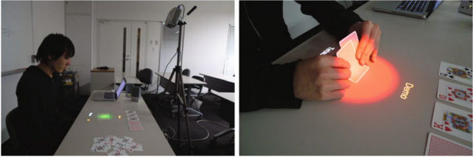
Fig. 4. EmoPoker system and visual feedback example. The projector spotlights the player’s hand cards and the color indicates arousal level (e.g., blue: calm, red: aroused). RFID tags are attached to each card in an unobtrusive way so that poker game events can be implicitly tracked and recorded by the system.
