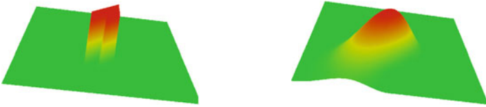
Fig. 2 Left: characteristic coarse grid basis function. Right: smooth coarse grid basis function
