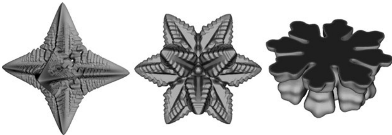
Fig. 4 Sample simulations of dendritic crystal growth with (from left to right) 4-fold, 6-fold crystalline anisotropy and a cut through an 8-fold crystal
