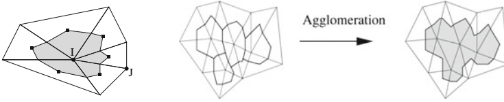
Fig. 1 Left: finite-Volume partition built as dual of a triangulation. Right: Greedy Algorithm for finite-volume cell agglomeration: four fine cells (left) are grouped into a coarse cell
