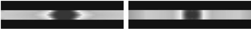
Fig. 4 Gas saturation at the end of the gas injection. Section y = 25 m . Farthest to the well : S = 0 . Closest to the well : S = 1 . Left: TPFA scheme. Right: VAG scheme
