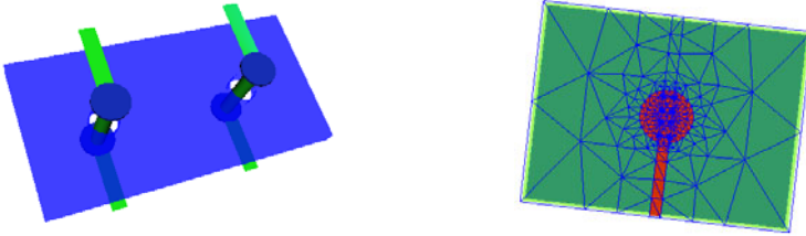
Fig. 1. (a) Coupled “through hole” via structure (b) 2D meshing for single via structure (Courtesy of Cadence Design Systems)
