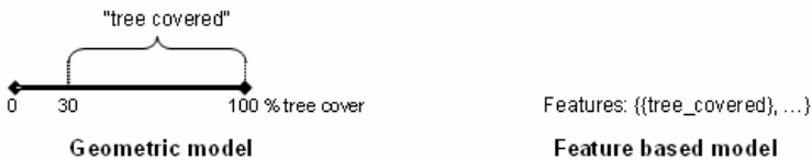
Fig. 1. The descriptive characteristic “tree covered” represented in a continuous geometric model (left) and a Boolean feature based model (right)
