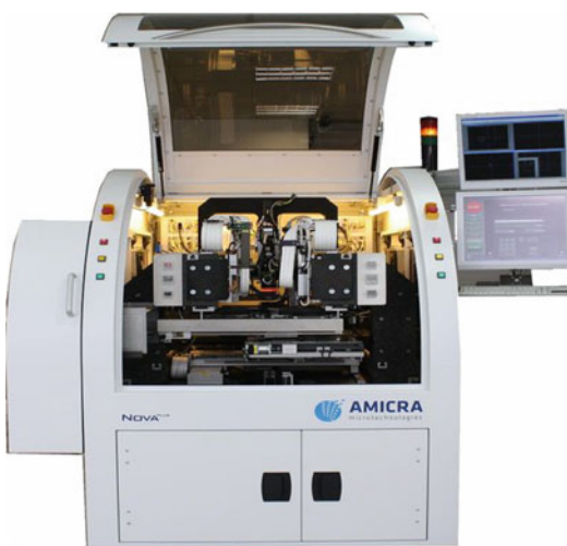
Eutectic Bonding, Fig. 3 High speed dual head die bonder (Amicra)
