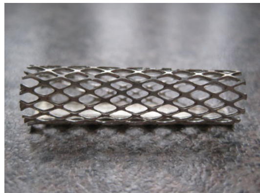
Etching, Fig. 5 Prototype cylindrical magnesium stent
