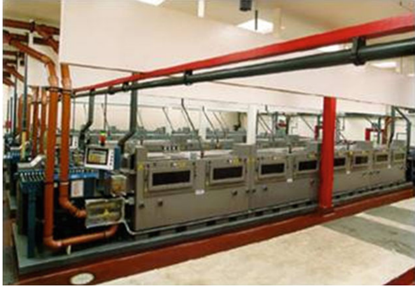
Etching, Fig. 1 Spray etching machines (Courtesy of PrecisionMicro, Birmingham)
