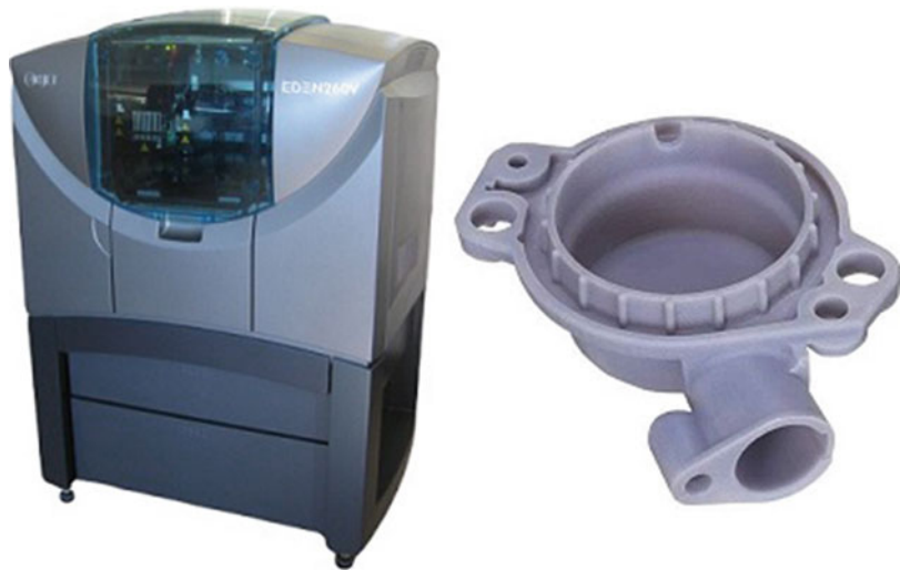
Fig. 8 Objet Eden 260v with a demonstration part (Material: Objet VeroBlue®)
