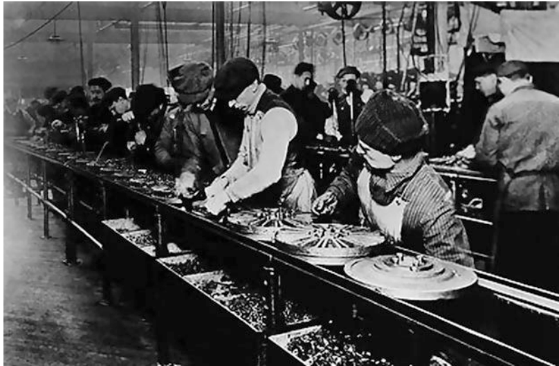
Assembly Line, Fig. 2 Assembly of the flywheel magneto for the T Model at Ford (Shimokawa 1997)
