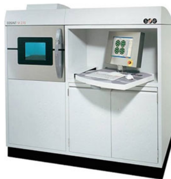
Fig. 12 EOS EOSINT M280 with demonstration parts (Material: EOS MS1®)
