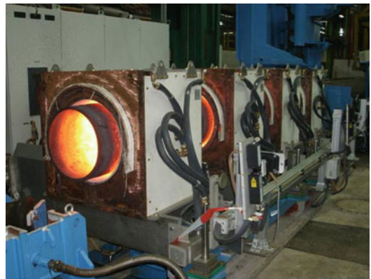
Induction Heating, Fig. 10 Inductive heating of a tube right before hot forming (Source: ITG Induktionsanlagen GmbH)
