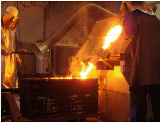
Induction Heating, Fig. 7 Induction furnace for 300 kg steel during casting (Source: ITG Induktionsanlagen GmbH)
