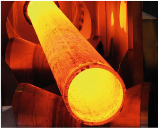
Induction Heating, Fig. 6 Hardening and tempering of a tube (Source: ITG Induktionsanlagen GmbH)
