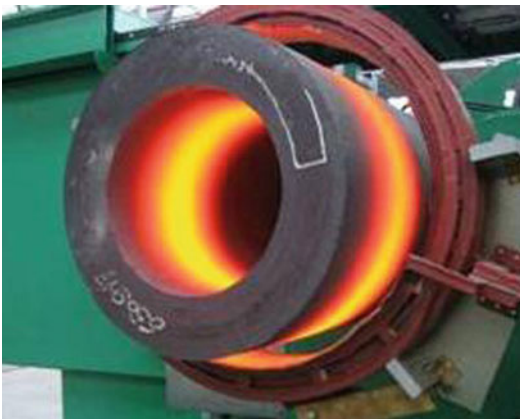
Induction Heating, Fig. 8 Induction coil on a tube bending machine (Source: ITG Induktionsanlagen GmbH)
