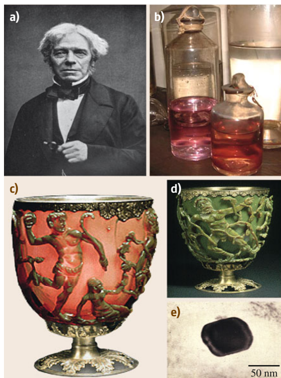
Fig. 9.1 (a) Michael Faraday (after [9.3]). (b) Faraday's gold preserved at the Royal Institution of Great Britain (after [9.4]). (c,d) The Lycurgus cup made from glass appears red in transmitted light and green in reflected light (after [9.5]). (e) The 70 nm Au-Ag alloy NPs found in the glass of the Lycurgus cup, as seen in a transmission electron micrograph (after [9.5])
