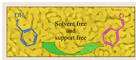
Fig. 21.18 NPG shows high selectivity and conversion for gas-phase selective oxidation of benzyl alcohol to benzaldehyde (after [21.121])
