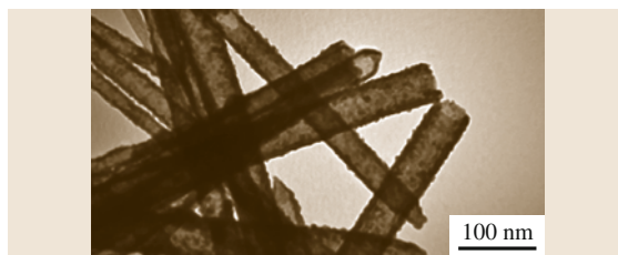
Fig. 10.11 CuPd bimetallic nanotubes prepared by galvanic exchange reaction on Cu nanowires. (After [10.232])
