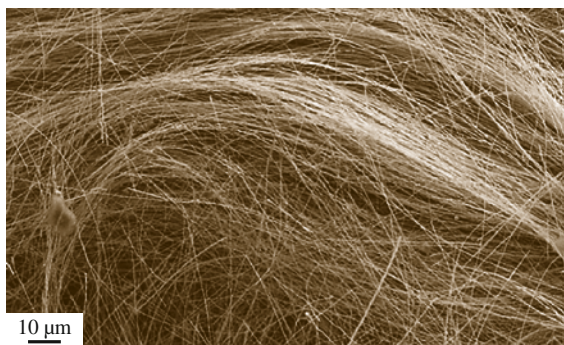
Fig. 10.6 Tungsten nanowires prepared by directional solidification and electrochemical processing of NiAl-W eutectic alloy. (After [10.140], courtesy of Wiley-VCH)
