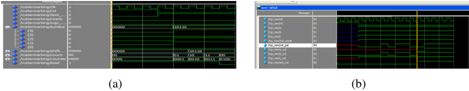
Fig. 3. (a) WGCResponse (when clock=1, reset=0 test mode=1 and ready signal =1). (b) Watermark sequence and test circuit response
