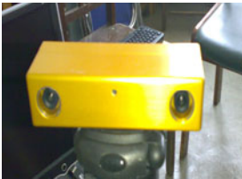
Fig. 5. Stereo vision camera Bumblebee2 Fig. 6. Image pair obtained by two cameras
