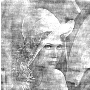
(c) Image obtained by taking the inverse Fourier transform from the synthesized spectrum (magnitude of the “Airplane” original spectrum and phase of the “Lena” original spectrum)
