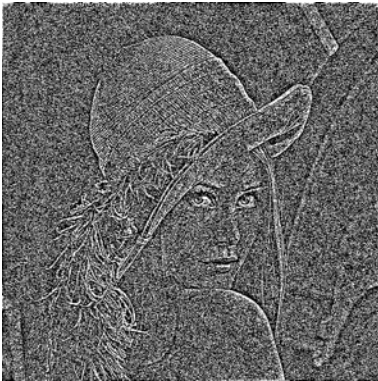
a) Image obtained by taking the inverse Fourier transform from the synthesized spectrum (“unitary” magnitude (constant 1) and phase of the “Lena” original spectrum)
