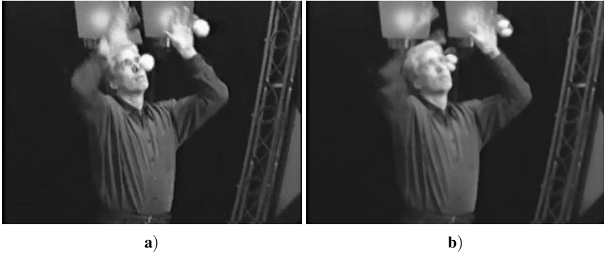
Fig. 2 Frame from popular Juggling video sequence and the result of temporal three dimensional Vector Median Filtering (processing window: 3 \times 3 \times 3 , norm L_1 ).
