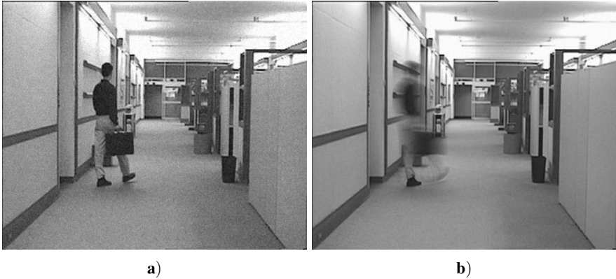
Fig. 1 Frame from standard video sequence hall monitor with additional Gaussian noise added ( \sigma = 10 ) and the result of temporal averaging with window length n = 9 .
