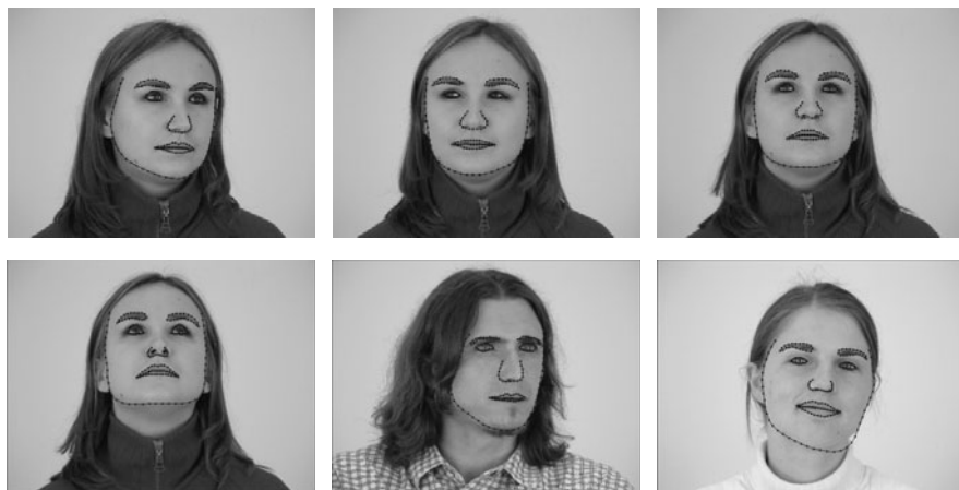
Fig. 5 Contours from LSN (top row) and TBS (bottom row) fitted by ASM
