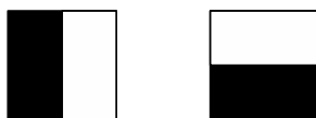
Fig. 1 Haar wavelets used to compute the gradient in the x and y directions, respectively. The weights are equal to 1 for the white areas, and -1 for the black areas.
