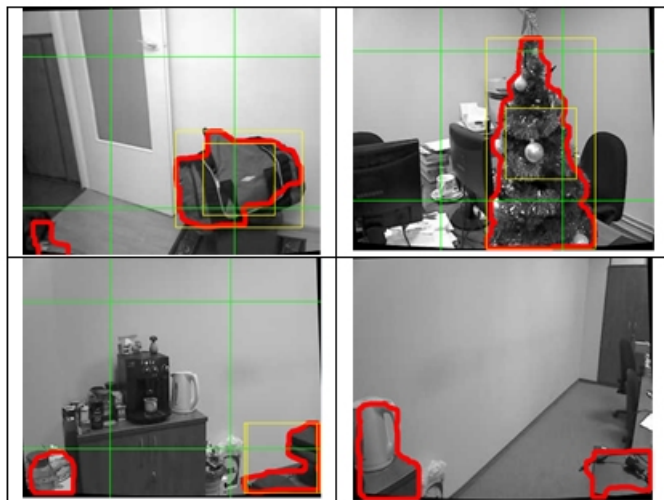
Fig. 5 Nearest obstacles detection and labeling (red line)
