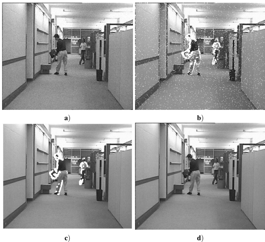
Fig. 3 a) Frame from standard video sequence hall monitor with additional Gaussian noise added ( \sigma = 10 ), b) Temporal Gaussian filtering with mask of skipped pixels, c) mask of skipped pixels after morphological opening (with mask of size 3 \times 3 ) and d) Final filtering result ( n = 5, \sigma = 5, \varepsilon = 11, \beta = 15 ).
