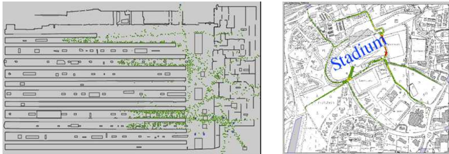
Fig. 4 Simulation of pedestrian traffic in a railway station and of a virtual regional evacuation of a stadium (Fritz Walter Stadium Kaiserslautern / Betzenberg). Pedestrian flows are reproduced in a natural way following the shortest path to the exits instead of following grid directions .
