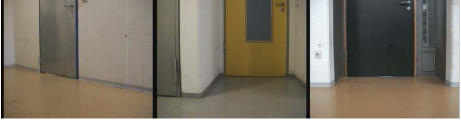
Fig. 1. Illustrates typical door images, taken by the robots camera. The top of the doors are cut off and also the diversity of doors are recognizable: The doors have different poses, colors, lighting situations as well as different features e.g. door gap or texture on the bottom.
