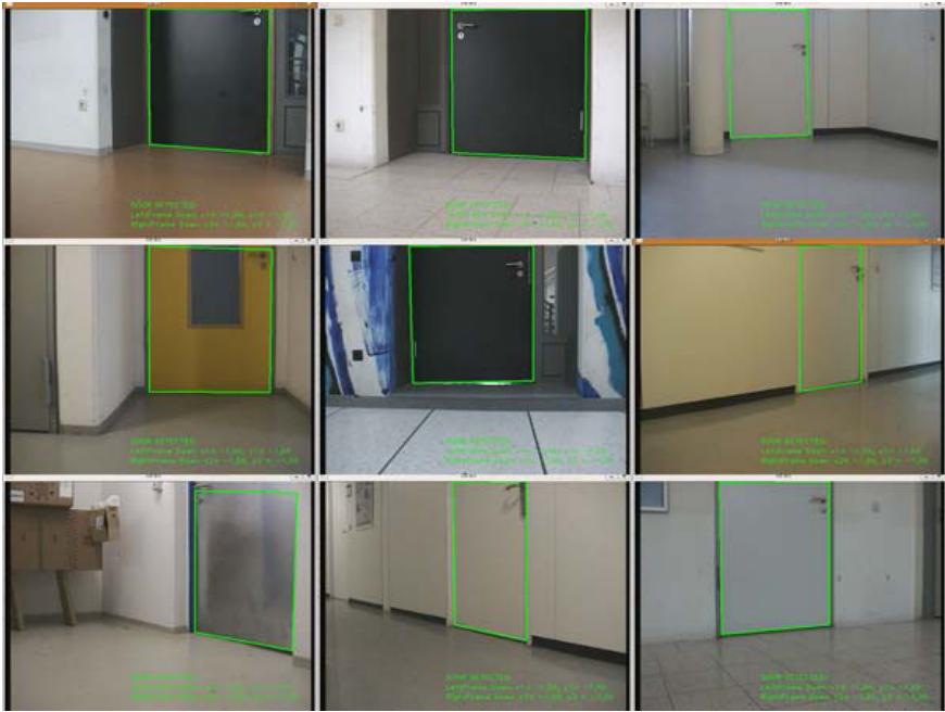
Fig. 7. These are typical examples of AdaBoost classifier detected doors. The pictures demonstrate that our approach is robust against different robot positions, reflection situation as well as different door features.
