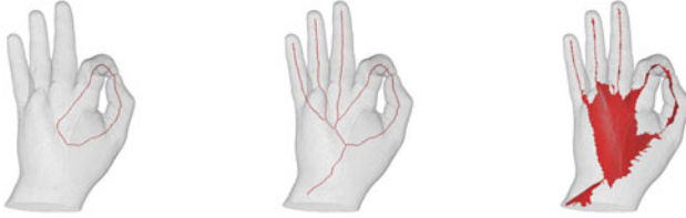
Fig. 1. From the left to the right (in red):ultimate, curve and surface skeletons
