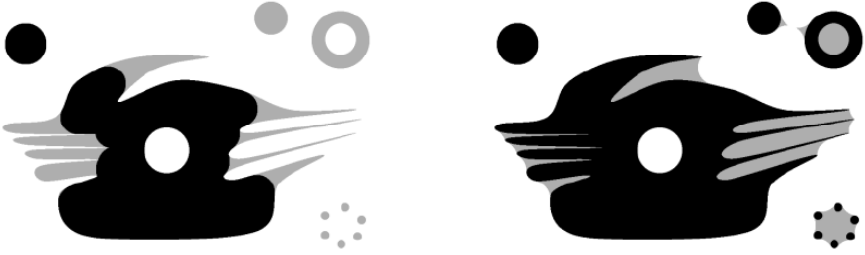
Fig. 2. On the left, we show the result R_r(S) of rounding in black and the material S - R_r(S) removed by the rounding operation in grey. On the right, we show S in black and the material F_r(S) - S added by filleting in grey.
