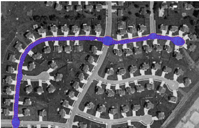
Fig. 18. A particular street is traced by Pearling in real-time. Upon request, the tracing may expand to branching streets.
