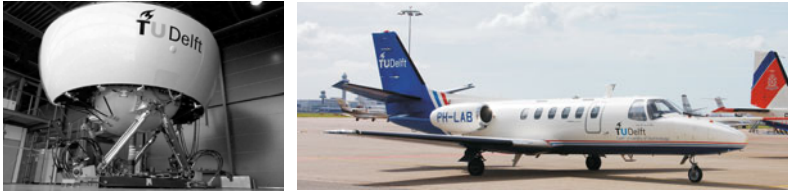
Fig. 4 SIMONA Research Simulator and Citation II laboratory aircraft of the Delft University of Technology.
