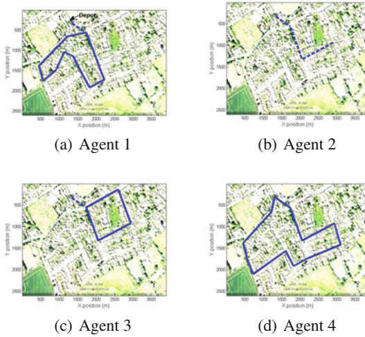
Fig. 3 Search path result of cluster algorithm. Solid line is vehicle path visited once and dashed line is duplicated vehicle path.
