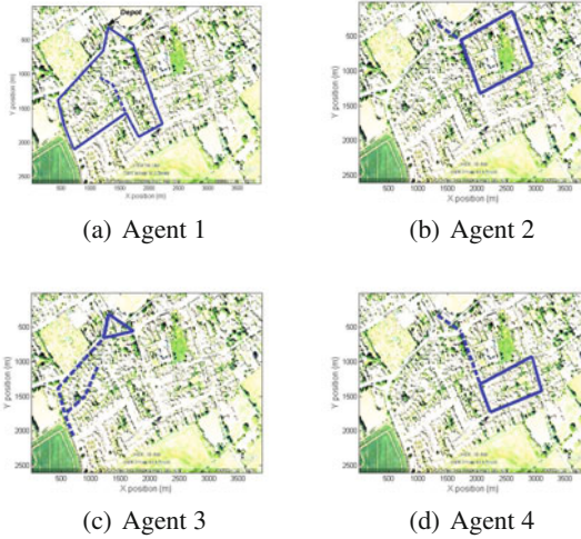
Fig. 2 Search path result of the cluster algorithm. Solid line is vehicle path visited once and dashed line is duplicated vehicle path.
