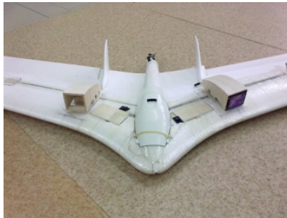
Fig. 16 The testing airframe – delta wing MAV
