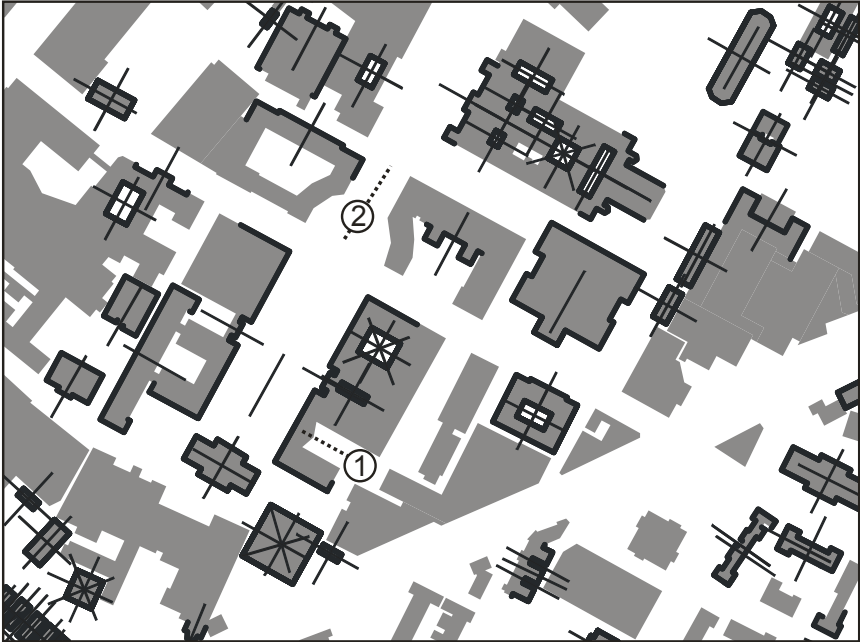
Fig. 9. Detected mirror axes (thin continuous lines) and corresponding building parts (bold lines) for the sample in Figure 3. The dashed lines labeled with (1) and (2) display axes that were not detected.
