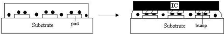
Fig. 1. Schematic figure of ACF bonding processing
