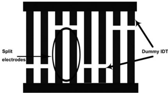
Fig. 4. Split electrodes and dummy IDT
