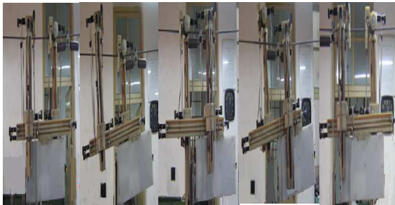
Fig. 7. Figures of inspection robot to cross overhung counterweigh autonomously
