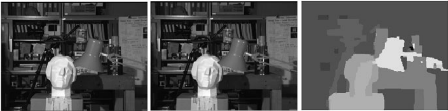
Fig. 2. Left/Middle: Images of Tsukuba stereo set; Right: Computed disparity map using our implementation
