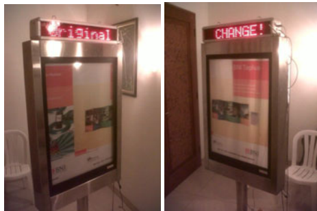
Fig. 5. New message (right) replacing the old message (left) in the billboard after it is changed from a notebook
