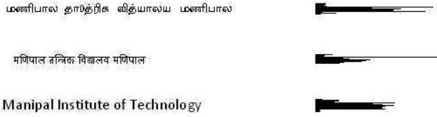
Fig. 1. Horizontal Projection Profile of a sample document with all 3 scripts
